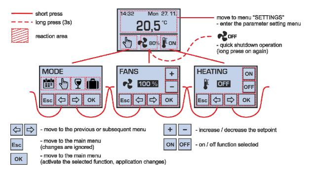
If operation is switched off by setting the ventilation capacity to "OFF", the unit does not respond to external requests, i.e. switches in the bathroom, toilet and kitchen and the air quality sensor are ignored.
