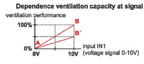
Setting the "inversion" response of ventilation capacity control to the 0-10V control signal (i.e. the opposite slope of the A - B curve).
