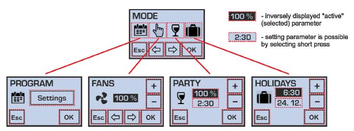
If more parameters are shown in the menu, you can switch between them by a short press; the value of a parameter can then be set by repeatedly pressing the "+" and "-" symbols (setting is faster if a symbol is held).
